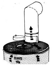
Open the smoke damper and draw the ash box open for 5-10 cm. See that sufficiently combustion air comes into the sauna either from the valve or through the door. Note that the sauna is not ready for bathing until the
