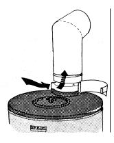
If there is no ventilation valve in the upper part of the sauna, the sauna can when necessary be ventilated by closing the löyly shutter and by opening the flap in front of the smoke damper. This can also be used for drying the sauna after bathing. The smoke damper must then be shut (picture).
